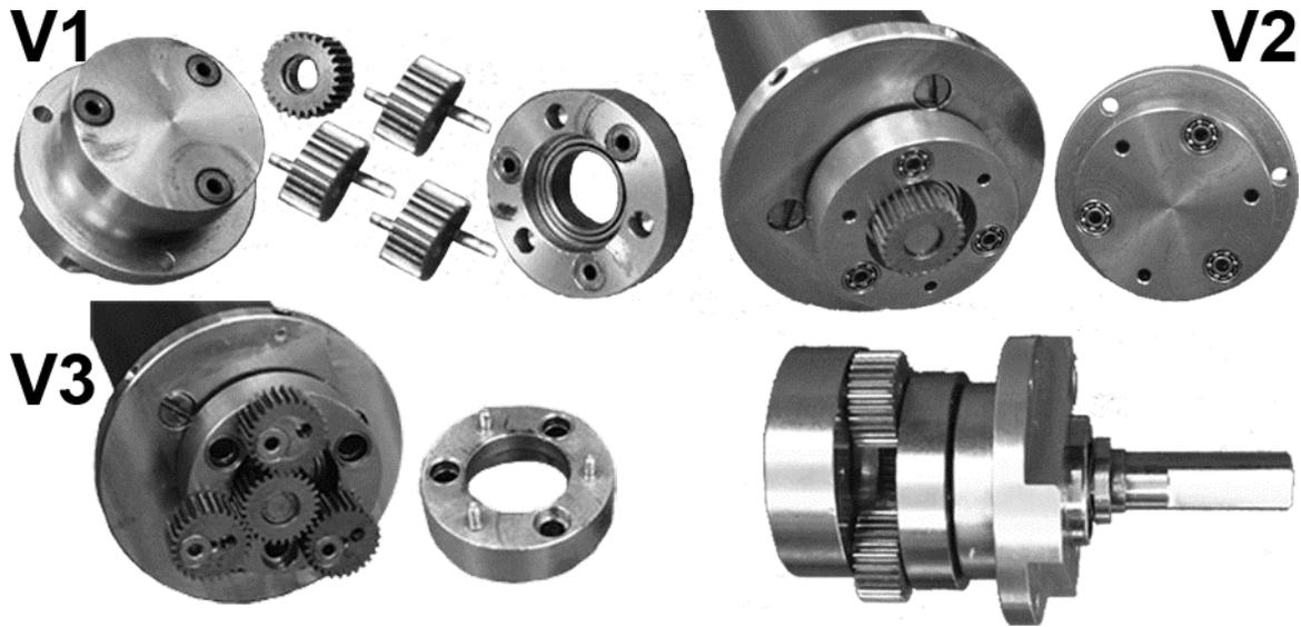
Fig. 3: Version 1, 2 & 3 Orbitless Prototype Gear-Head
