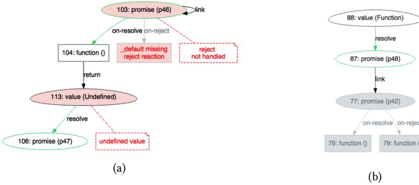
Fig. 10. Examples of missing reject reaction, Telegraph (10a) & unreachable reaction, Serialport (10b).
